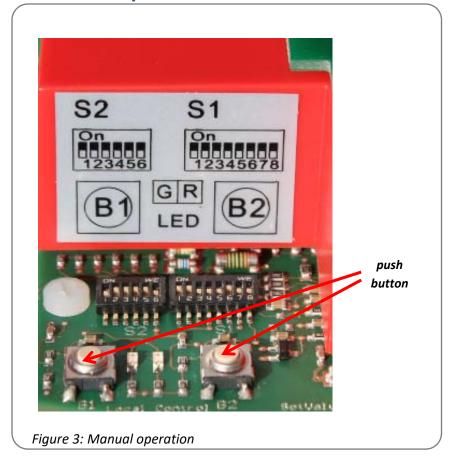
Two push buttons are installed to drive the actuator in case of installation work such as mounting onto a valve, or setting the limit switches positions (see 10.7).
