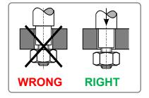
Before the pillar nuts are tightened, make sure that the pillars are sitting on the valve mounting base. If necessary, correct the position of the actuator by using manual operation. If these instructions are not observed, personal injury or damage to the actuator and/or valve may result.
